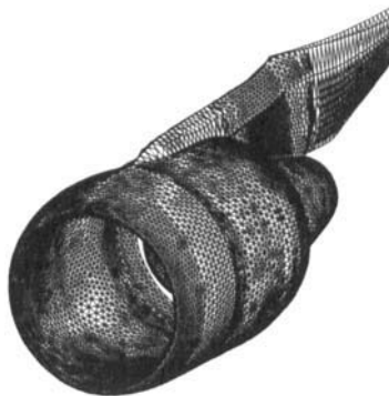
Figure 3. Grid on the surface of a nacelle generated using the Delaunay triangulation and the automatic point creation algorithm
